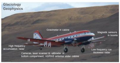
EMR, accumulation and snow thickness radar, ultra wide-band radar, mUWB, gravimeter, magnetometer, ASIRAS (ESA), EM bird, laser scanner, long range laser altimeter
